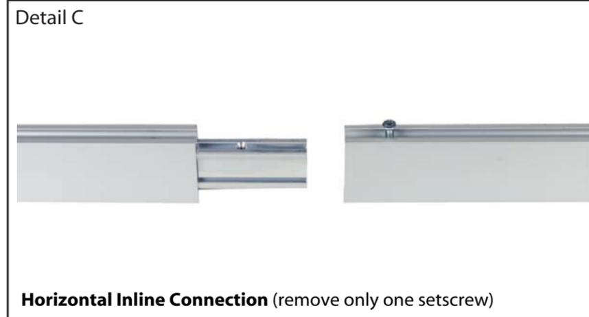
**Horizontal Inline Connection** (remove only one setscrew)
