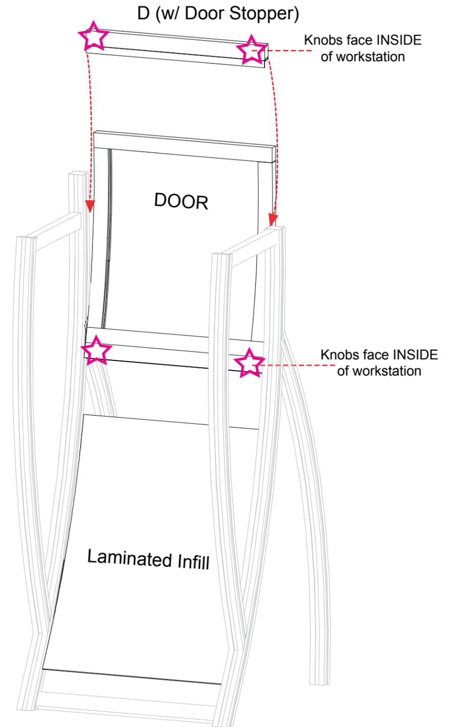
**WHEN DISASSEMBLING TIGHTEN ALL KNOBS TO PREVENT LOSS DURING SHIPPING**
