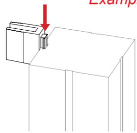
When desired location is found, tighten set screw to secure.
