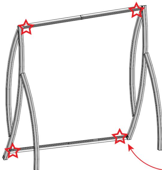
STAR indicates location of knobs on BACKSIDE of unit.
