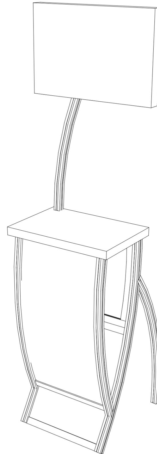
WHEN DISASSEMBLING ALUMINUM EXTRUSION, TIGHTEN ALL SETSCREWS AND LOCKS TO PREVENT LOSS DURING SHIPPING
