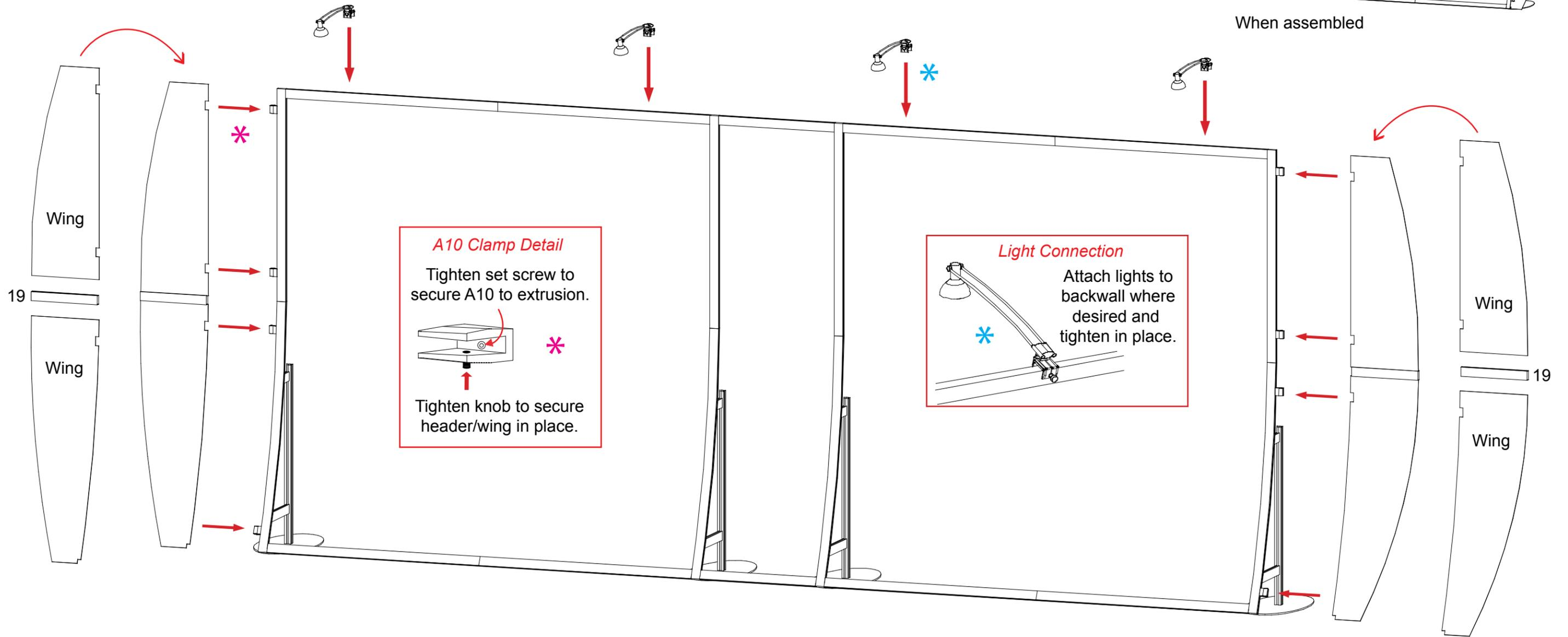
**WHEN DISASSEMBLING ALUMINUM EXTRUSION, TIGHTEN ALL SETSCREWS AND LOCKS TO PREVENT LOSS DURING SHIPPING**
