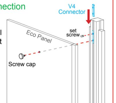
Attach Eco Panel to V4 connector using screw caps.
