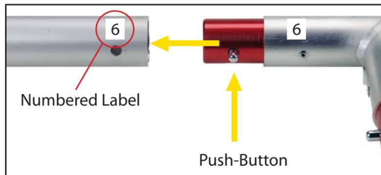
Connections are made by holding the button down and sliding the red tube into opposing tube until the connection is made. To disassemble push button and pull or twist extrusions apart.
