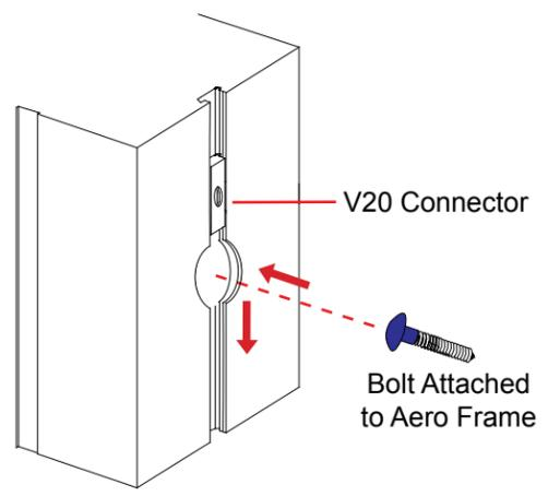
Insert bolts of aero frame into keyhole slot in groove of vertical extrusion, slide aero frame down to secure.
