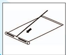
Assemble pole and place into base locking onto pin inside base.
